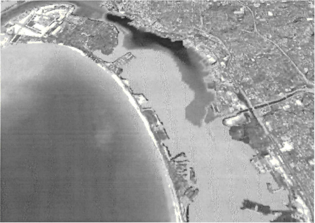
Figure 6. Bayview depiction of stormdrain and creek output using coupled watershed and hydrodynamic models. A panchromatic SPOT image is overlaid on U.S. Geological Survey digital elevation data. Bathymetry is provided by the U.S. Navy.
