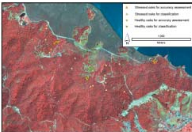
Figure 2 ADAR imagery (false color transformation (4,3,2)) of the study area. Ground control points are superimposed on the imagery.
