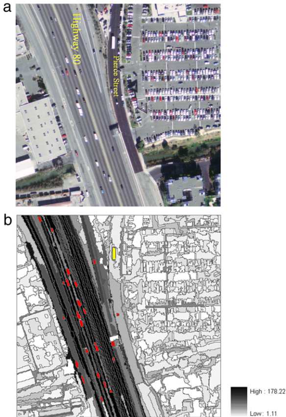
Fig. 11. (a) The original image and (b) the segmented result, where the grey scale of each object represents its relative longness index (RLI), and the extracted moving vehicles are shown in red.
