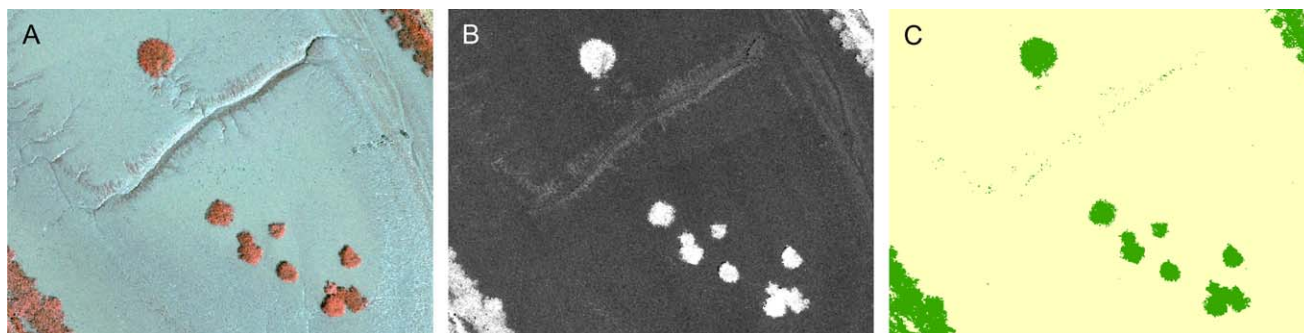
Figure 2. Each CIR image (A) was transformed to NDVI (B), after which pixels were reclassified as vegetated or nonvegetated (C).
